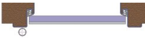
Horizontal fitting outside face
